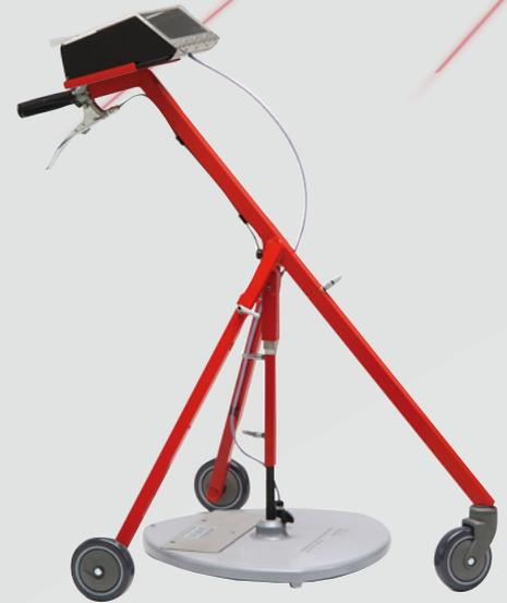
statistical evaluation of material thickness variations caused by uneven pavements, wearing, deformation or other important factors impairing road layer material quality.
