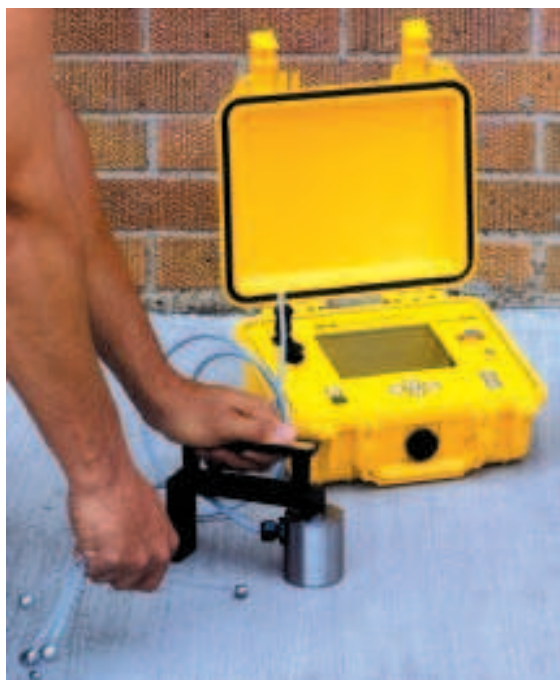
Measuring the quality of a concrete slab with the Vu-Con System
