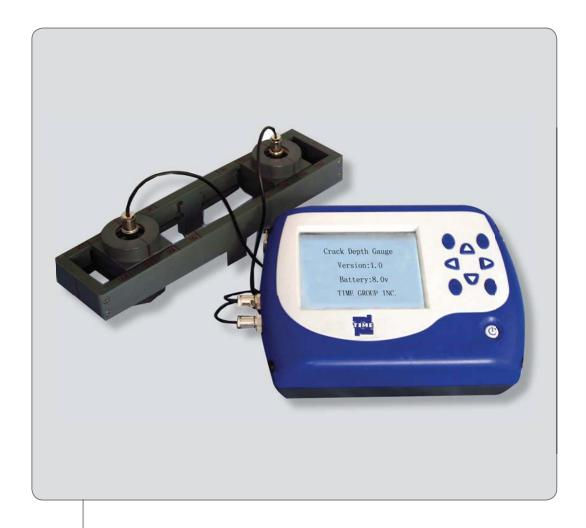
**TC200** is used to measure concrete crack depth by applying principle of acoustic diffraction. At the same time, it is also used to measure propagation velocity of ultrasonic wave in concrete. This instrument is a kind of intelligent nondestructive test equipment possessing the functions of automatic detection, data memory and output.
