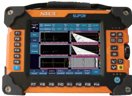
PA & TOFD with Conventional UT
