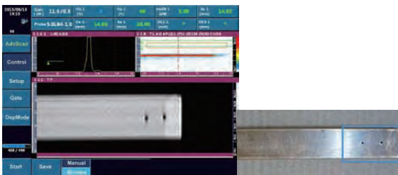
● C-scan on copper bar with two \phi 1 short cross-drilled holes (depth: 0.5mm)
