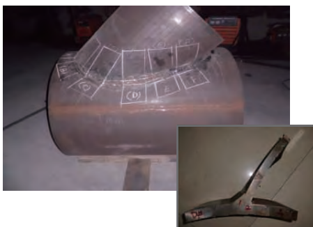
Y-shape weld joints cut from a huge pipe
