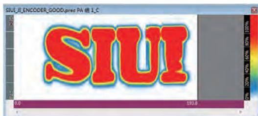
C Scan In-Amplitude, showing echo amplitude
